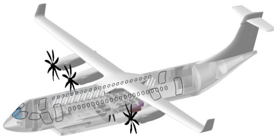
Figure 6. Batteries installation into 80-pax aircraft belly.
