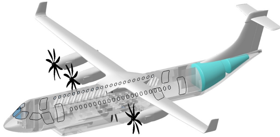
Figure 11. Tanks installation within the NEWBORN 80-pax aircraft.
